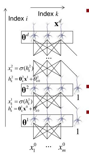
Forward propagation per layer in matrix notation:
