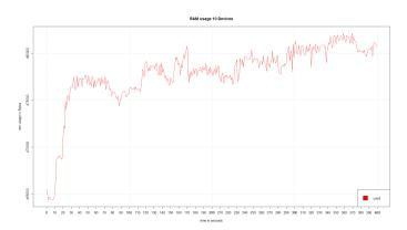
Fig. 5. RAM Usage on the edge node: Starting 10 Devices
