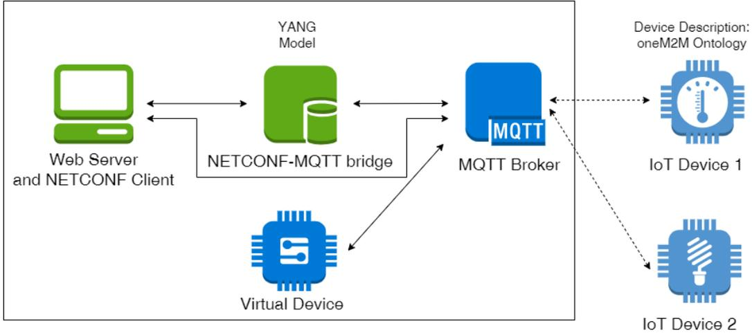
Fig. 2. MYNO System Architecture
