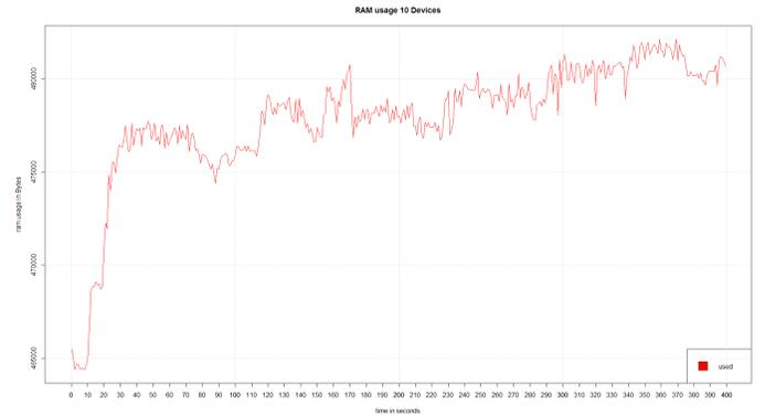
Fig. 5. RAM Usage on the edge node: Starting 10 Devices
