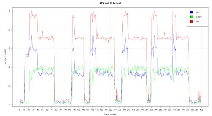
Fig. 4. CPU Load on the edge node: Starting 10 Devices.
