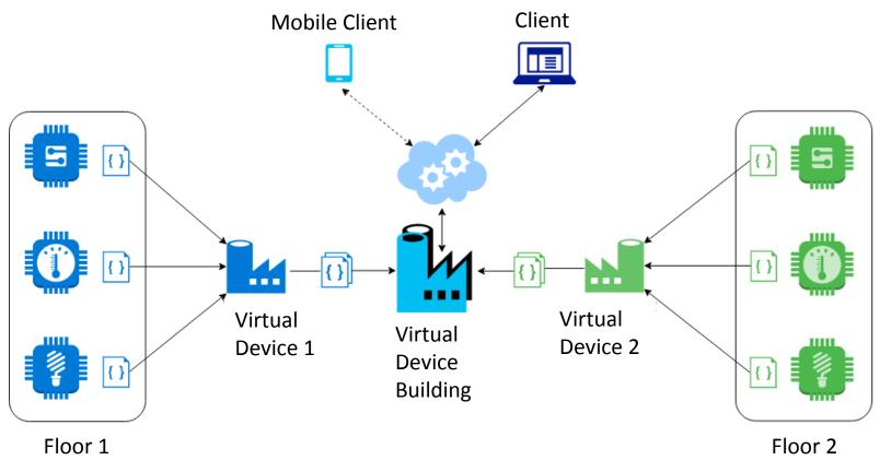
Ontology-based Virtual IoT Devices for Edge Computing
