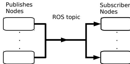
Fig. 1: ROS topics provide many-to-many asynchronous message passing.
