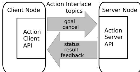
Fig. 2: ROS actions provide preemptible client-server communications.
