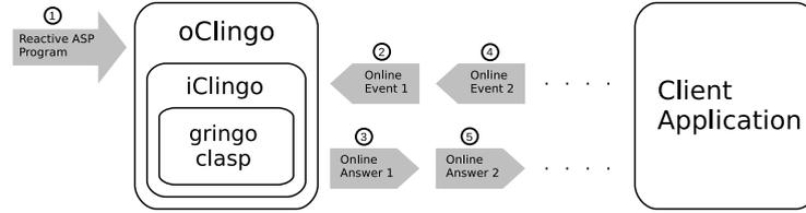
Fig. 4: Basic workflow between oClingo and a client application.
