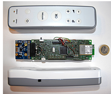
Fig. 3. The Figure shows the EasyReach remote control, its keyboard and enclosure and its internal electronics
