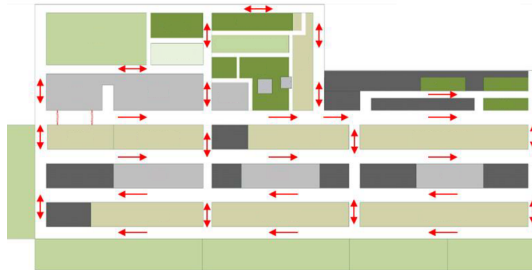
Fig. 1. Real-world factory layout with transport corridors and directions indicated by arrows
