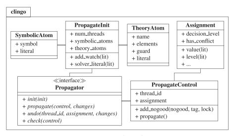
Fig. 3. Class diagram of *clingo*'s (theory) propagator interface.
